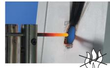
Burning behaviour: Glow wire test according to IEC 60 695-2-11: 750 °C, flame-retardant, self-extinguishing
