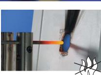
Burning behaviour: Glow wire test according to IEC 60 695-2-11: 750 °C, flame-retardant, self-extinguishing
