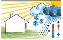
Here condensed water can be formed dependent on the weather, high air humidity, direct sunlight and temperature differences compared to the wall.
