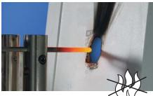
Burning behaviour: Glow wire test according to IEC 60 695-2-11: 750 °C, flame-retardant, self-extinguishing
