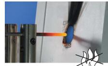
Burning behaviour: Glow wire test according to IEC 60 695-2-11: 960 °C, flame-retardant, self-extinguishing
